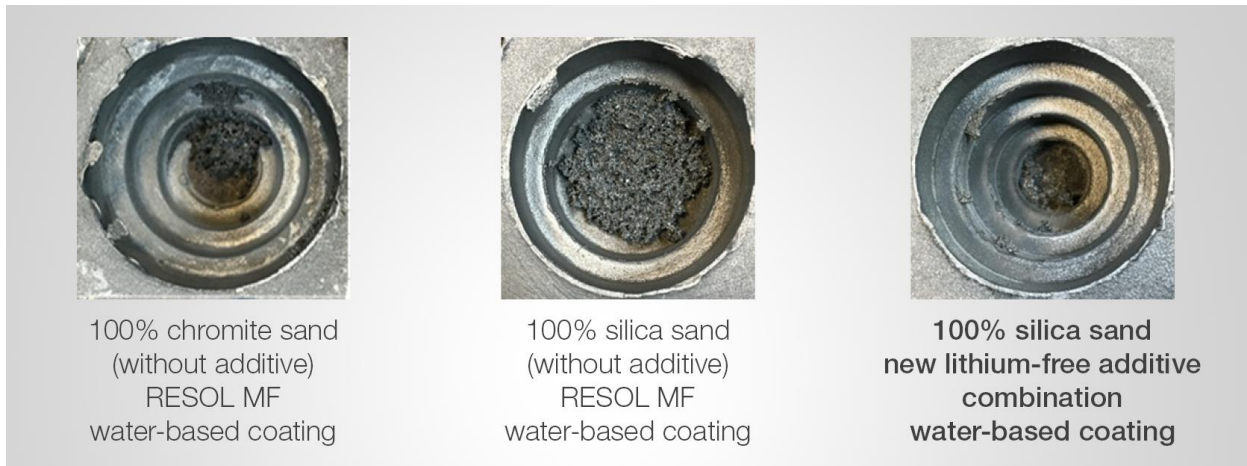
Fig. 8: small step cones, GJL, casting temperature approx. 1420 °C, water-based coating ( ASK Chemicals )
