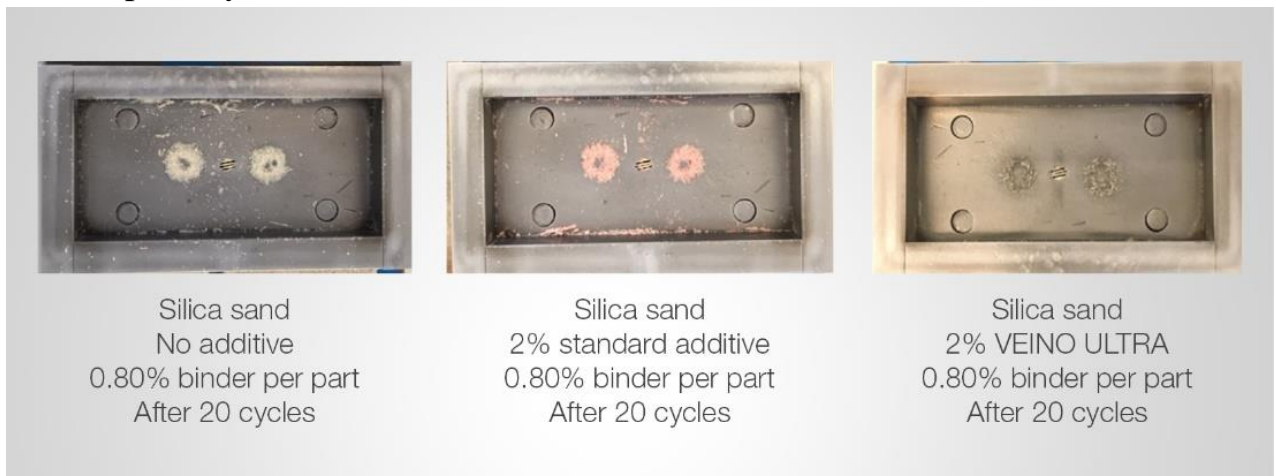
Fig. 3: Core box; comparison of sand additive and binder buildup (cold box) underneath of two inserts. Result after 20 cycles and without release agent application, lab test ( ASK Chemicals )
